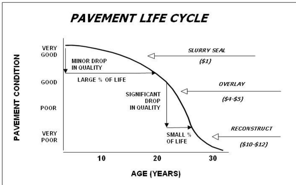
Figure 5: Degradation Curve<sup>4</sup>
